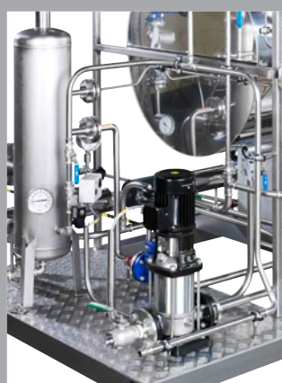
Pressure booster system and liquid waste removal filter
